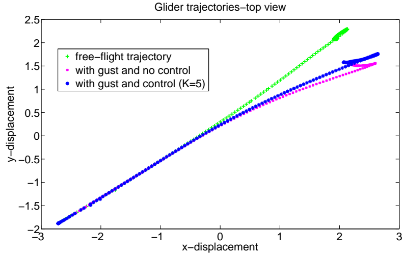
Figure 4.14: Glider trajectories: in free flight, under the influence of a gust and using strain feedback.
