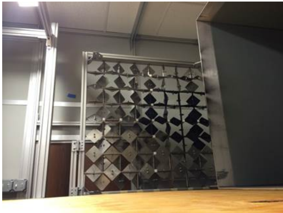
Figure B.1: ATG turbulence grid
